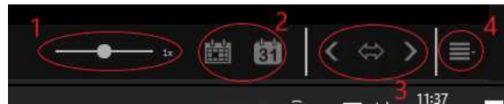
1. playback speed 2. select whole current day and calendar 3. timebar movement buttons and expand time button ( also includes hover note with mouse control binding information ) 4. additional playback functions menu
