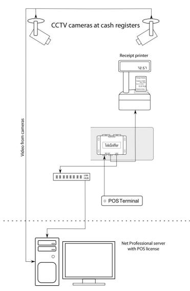
Alnet sniffer is connected through serial ports between cash register and printer. It allows to capture transaction data transparently for both devices and transfer it in real time by TCP/IP protocol to main server with NET PROFFESIONAL running. Application with POS license displays transactions in real time on selected cameras and saves it to the database, for the future management (search, browse, selection). As a final outcome user gets list of transactions correlated with video stream.
