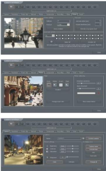
The Camera Configuration menu allows for the precise configuration of all camera parameters on all individual cameras. Multilevel menus allow for easy to understand tools that are available for each camera. Motion detection is one of the tools available in the camera configuration, where sensitivity and object masking are essential for each camera, especially for areas with constant motion.
