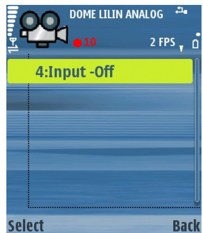
Picture16: Displaying the available alarm inputs
