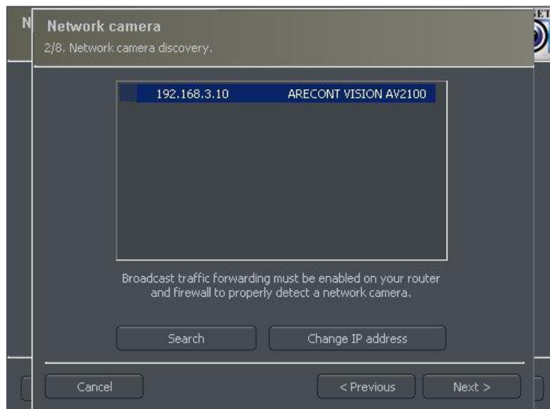
Figure 8 Search function automatically detects available network cameras. User can manually change camera IP address – Change IP address button.
