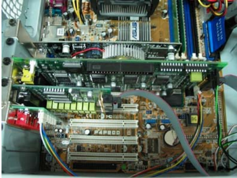
<AS3000V2, AudExt2 and ConExt1616 Inserted into PCI Slot>
