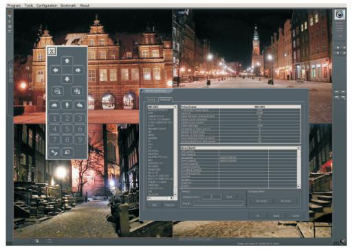
NetStation allows for the connection of up to 64 PTZ cameras. Controlling of the P/T/Z functions, can either be done manually using the keyboard, joystick, mouse or the on screen control panel. Wide range of supported domes made by several manufacturers, provide great compatibility. Preset Control is an option that can be set manually on PTZ cameras, so specific cameras can monitor larger areas.
