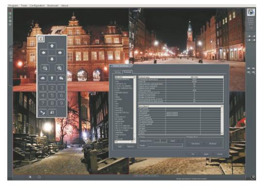
NetStation allows for the connection of up to 32 PTZ cameras. Controlling of the P/T/Z functions, can either be done manually using the keyboard, joystick, mouse or the on screen control panel. Wide range of supported domes made by several manufacturers, provide great compatibility. Preset Control is an option that can be set manually on PTZ cameras, so specific cameras can monitor larger areas.
